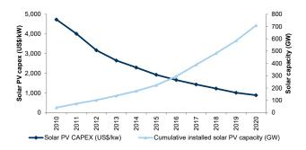
Solar PV capex (US\$/kW) vs. global cumulative solar PV capacity (GW)
