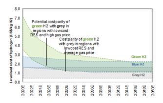
Exhibit 13: The unique dynamic in Europe with historically high gas and carbon prices is already leading to green H2 cost parity with grey across key parts of the region (LCOE <US\$50/MWh) Levelized cost of hydrogen - LCOH (US\$/kg H2)
