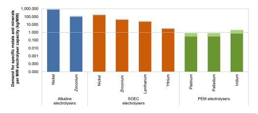
Demand for specific metals and minerals per MW electrolyzer capacity (kg/MW)
