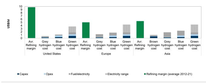
Refining margin and hydrogen cost per barrel (US\$/bl)
