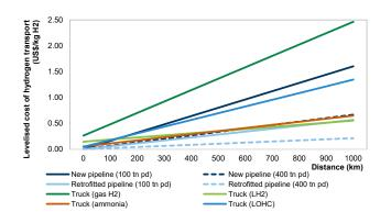
Exhibit 96: ..but pipelines (especially retrofitted) are the most economical solution for local and short-distance distribution/transmission once conversion/reconversion costs are considered
