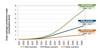
Exhibit 117: ...which, from a global perspective, is not very material, representing c.15% of the total energy sector's water consumption Water withdrawal (left) and consumption (right) for the energy sector and for clean hydrogen production under our GS hydrogen models (bcm)
