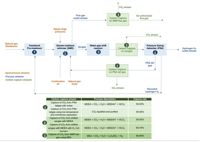
Exhibit 57: Schematic diagram presenting the steps of a typical 'blue' hydrogen production process combining SMR with carbon capture
